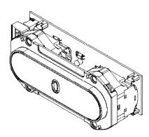
Compact 2 Bar Pushbuttons can be supplied loose or incorporated into stations with 1.5mm or 2.5mm stainless steel faceplates, with a vertical pitch of 65mm and horizontal pitch of 160mm i.e the pushbutton body can be rotated through 90 degrees (horizontal version shown above). If pushbuttons are supplied loose, spacers are provided to accommodate the differing faceplate thickness.
