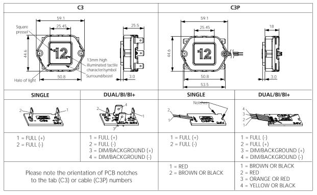
Compact 3/3P Pushbuttons can be supplied loose or incorporated into stations with 1.5mm or 2.5mm stainless steel faceplates, with a vertical pitch of 50mm and horizontal pitch of 60mm (C3) or 80mm (C3P) i.e the pushbutton body can be rotated through 90 degrees (horizontal version shown above). If pushbuttons are supplied loose, spacers are provided to accommodate the differing faceplate thickness.
