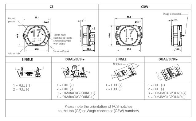
Compact 3/3W Pushbuttons can be supplied loose or incorporated into stations with 1.5mm or 2.5mm stainless steel faceplates, with a vertical pitch of 50mm and horizontal pitch of 60mm (C3) or 80mm (C3W) i.e the pushbutton body can be rotated through 90 degrees (horizontal version shown above). If pushbuttons are supplied loose, spacers are provided to accommodate the differing faceplate thickness.
